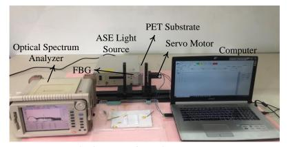
Fig. 4 Photo of experimental setup
